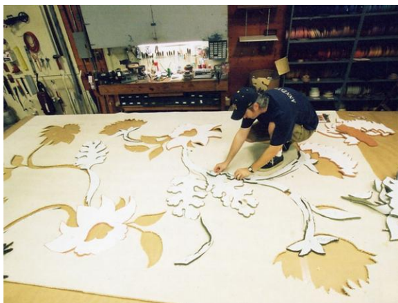
First, pieces are cut from carpet into the necessary shapes and put together like a puzzle.
