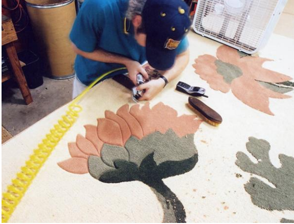
The rug is turned over and detailed with hand-shearing equipment.
